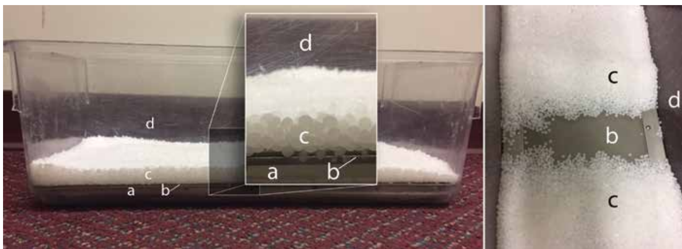
Figure 1. The synthetic bedding substrate (SBS) consists of (a) an absorbent pad below (b) a metal mesh screen that is custom-made to fit a large static cage, (c) polyurethane synthetic beads, and (d) a standard large mouse static cage. The concept is that moisture wicks over the beads, through the wire mesh, and absorbed by the underlying pad, thus keeping mice dry.
