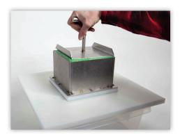
With the Gel Cutting Device plunger, push the gel squares through the blade assembly.
