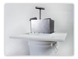
Set up the Gel Cutting Device on the Cutting Board placed over a bucket or storage container.
