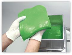
Place up to four gel squares into the Gel Cutting Device hopper.
