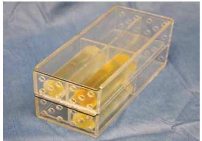
Figure 2. Acrylic mouse restraint box containing 3 phantoms. The box was portioned into 8 equal sections. Mice or acrylic phantoms (length, 3 in; diameter, 1 in.) were placed into each section.
