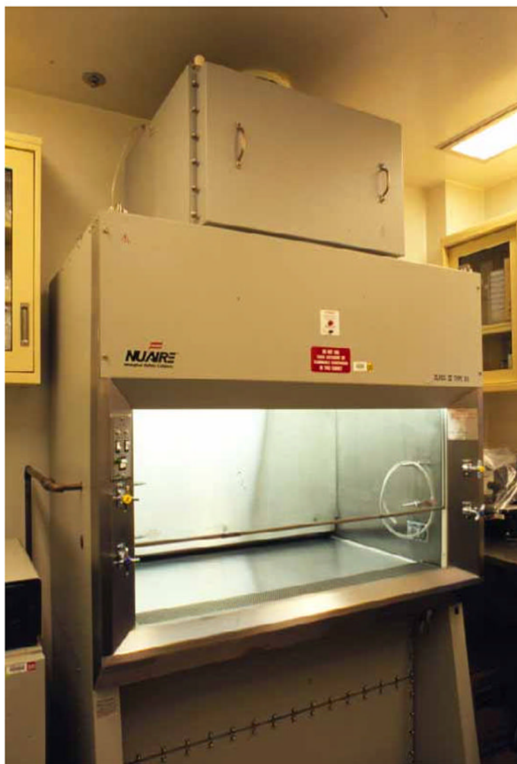
Figure 1.12.5. Type IIB biosafety cabinet.
