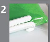
Using a Pouchmate opener, slice the pouch open and remove the gel square.
