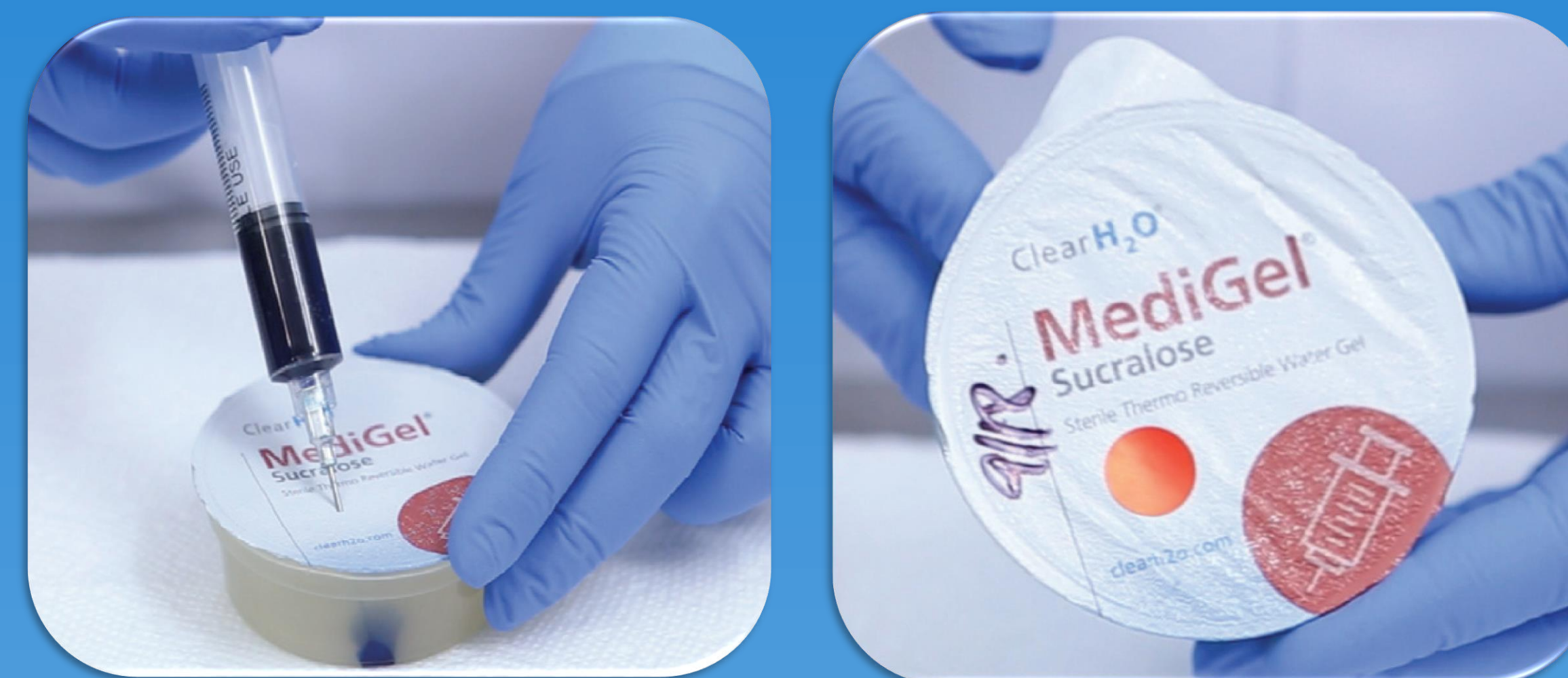
Figure 1. Gel in unopened cup was melted in a water bath (50-60 C°) and inoculated with dyed solution after wiping the lid with alcohol. The puncture in the lid was then covered with a sticker and the cup was dated.
