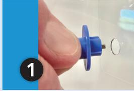
**1** Remove the cage lid and align the AquaValve<sup>®</sup> for insertion into the lid water access hole in the water bottle receptacle.
